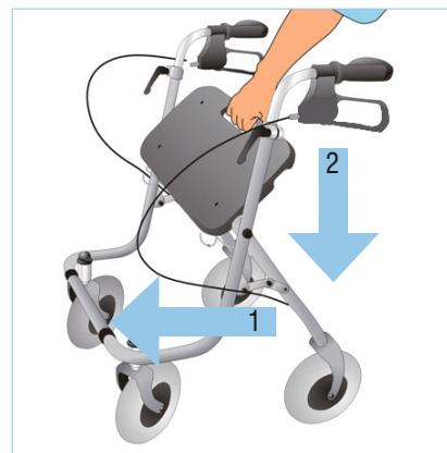
Position the walking device on its wheels. Push the front frame forward by pressing on the handgrips down and pulling backwards until the walking device stands on four wheels. Then press the seat down until it clicks into place on the crossbar.
